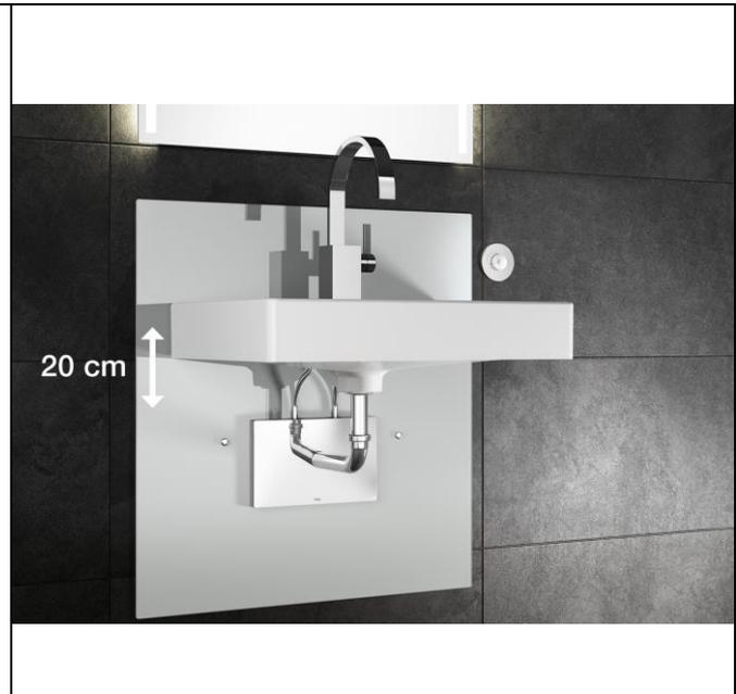
06: The sink element from Viega allows the sink to be continuously height-adjusted by 20 cm. At the press of a button, the unit independently moves up in a range between approximately 70 and 90 centimetres.
